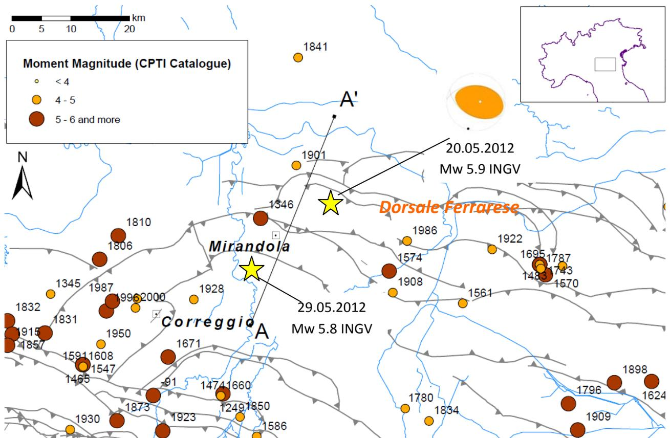
Fig 1: Capable faults, historical seismicity and drainage network in the epicentral area of the 20.05.2012 eq. (Michetti et al., 2012; modified); focal mechanism from NEIC; the trace of the geological section in Fig. 2 is also shown.
