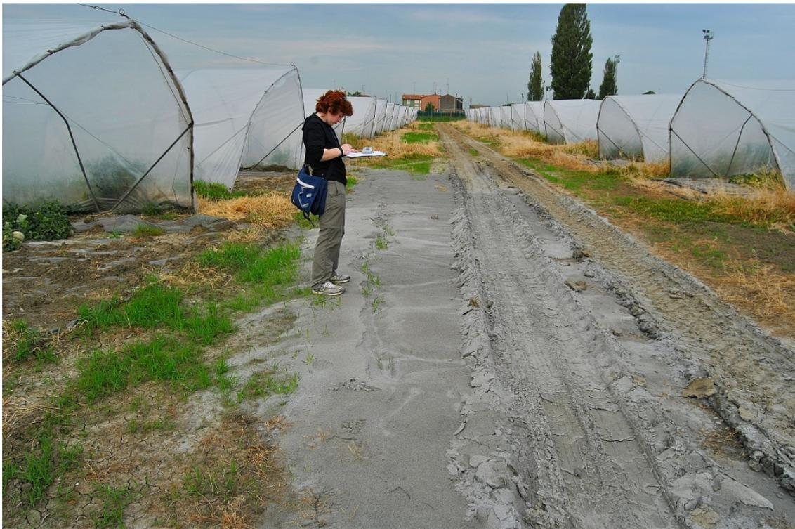
Fig. 6: Gavello, among the greenhouses ca. 25 fractures with gray-blue ejected sand have been mapped; photo taken on May 26, 2012.
