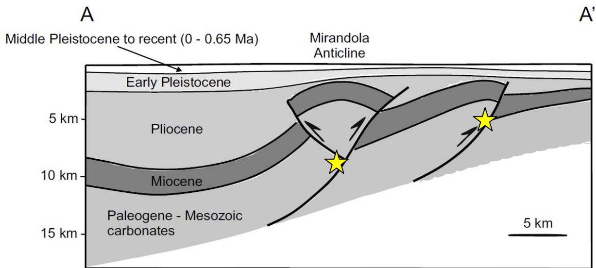
Fig. 2: Simplified cross section of the Mirandola structure, with very preliminary interpretation of the causative faults for the 20 and 29 May 2012 eqs. (Michetti et al., 2012; modified); the stars show tentative hypocentral locations.
